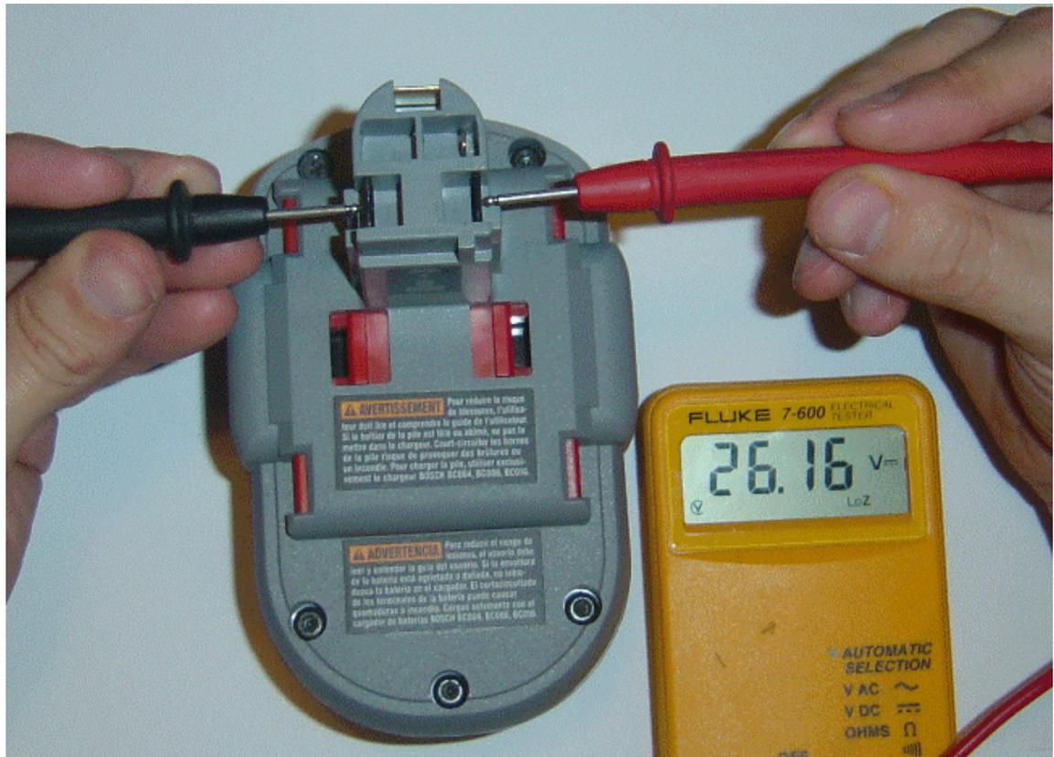
3) Take a reading on your Battery in question in DC volts. Write down the reading. Refer to this table for an explanation and suggestions.\*
